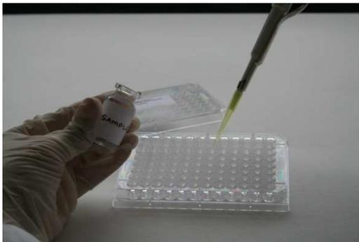
3. Obtain the sample or samples to be tested, and dispense and double dilute in the same manner as the control (again, row H is a reference row and Does not contain any sample materials).
