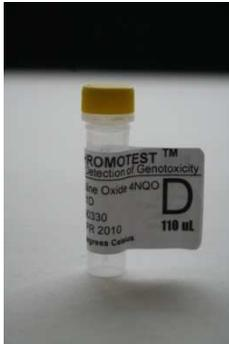
1. Obtain the 4NQO (Control) from the freezer, as well as all samples for assays. Dispense 20µl of the 4NQO solution into well 2A.
